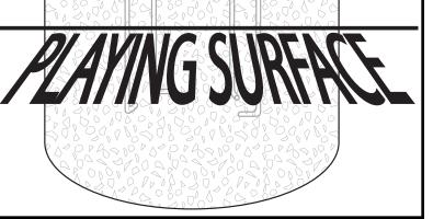
**IMPORTANT!:** WAIT A <u>MINIMUM</u> OF 72 HOURS BEFORE GOING ON TO NEXT STEP. CONCRETE <u>MUST</u> CURE. ALLOW ADDITIONAL TIME FOR COLD, WET OR HUMID WEATHER.
